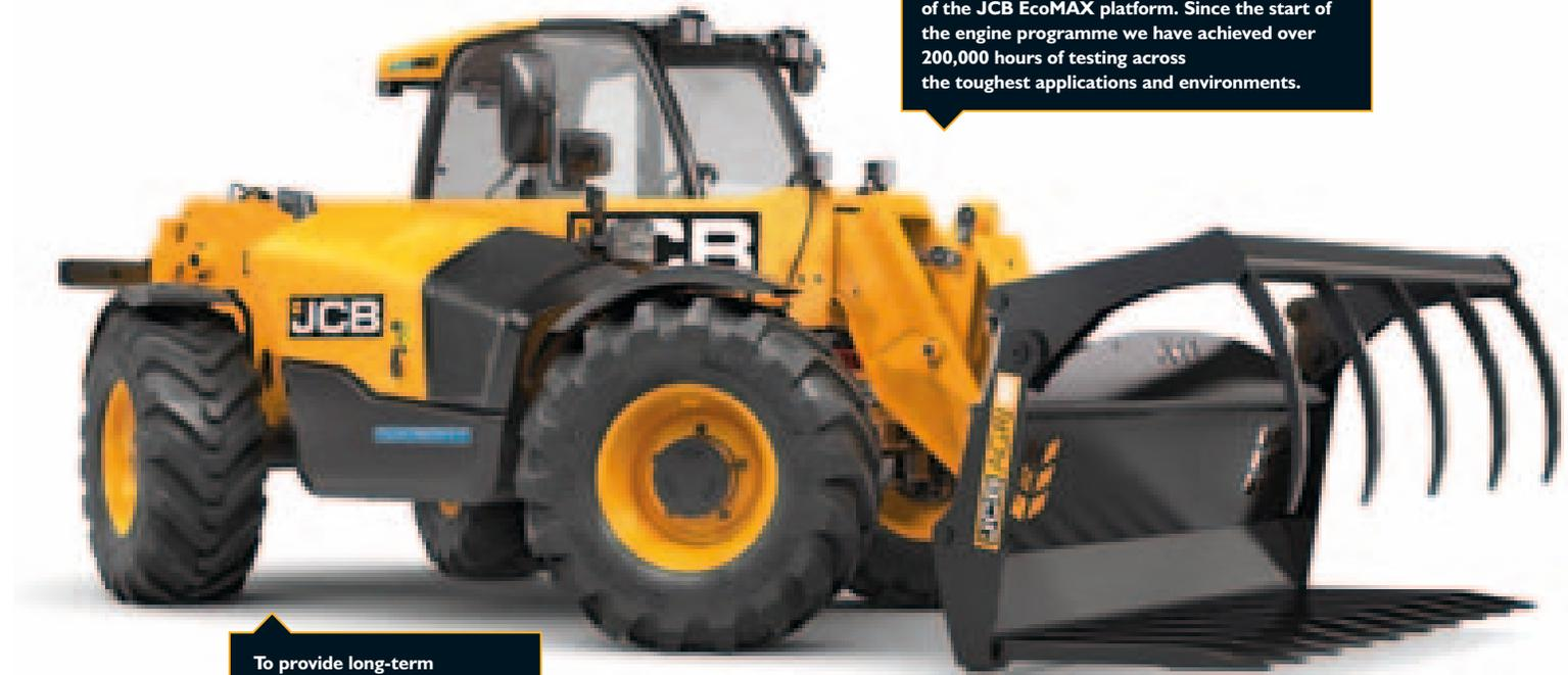
To provide long-term protection, we dip every AGRI Loadall cab in electrophoretic alloy before painting it.
