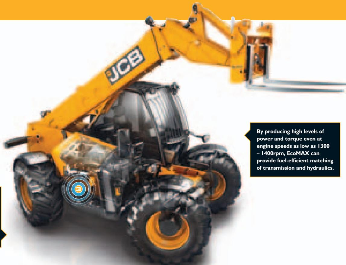
By producing high levels of power and torque even at engine speeds as low as 1300 – 1400rpm, EcoMAX can provide fuel-efficient matching of transmission and hydraulics.
