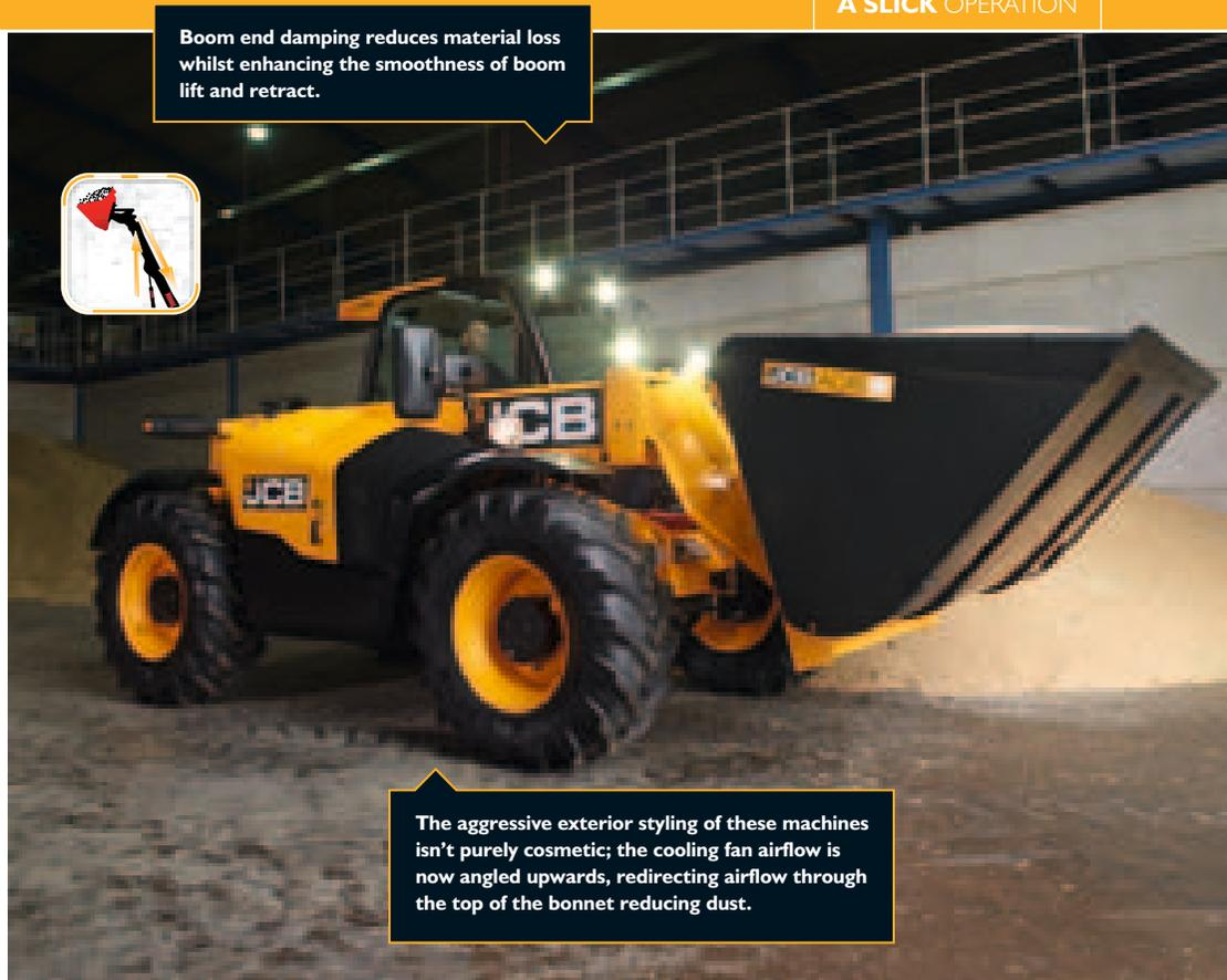
Boom end damping reduces material loss whilst enhancing the smoothness of boom lift and retract.
