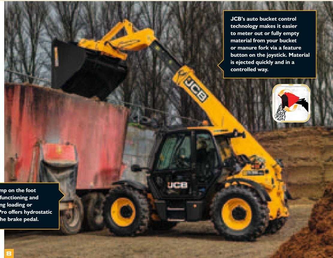
JCB's auto bucket control technology makes it easier to meter out or fully empty material from your bucket or manure fork via a feature button on the joystick. Material is ejected quickly and in a controlled way.
